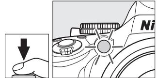
**Remote control mode:** From a distance of 5 m (16 ft.) or less, aim the transmitter on the ML-L3 at either of the infrared receivers on the camera (☐ 1, 2) and press the ML-L3 shutter-release button. *In delayed remote mode*, the self-timer lamp will light for about two seconds before the shutter is released. *In quick-response remote mode*, the self-timer lamp will flash after the shutter has been released.
